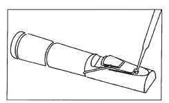
2. Place a drop of sample in the cover hole. Through capillary action it will disperse. Aim towards a light source to take reading.
