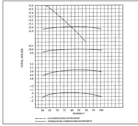
Figure 3 Temperature response of Model 1310400A TS METER
