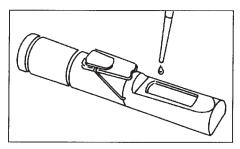
1. Place a drop or two of sample on the prism, close the cover and aim toward a light source or
