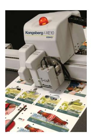
A Kongsberg i-XE table is a complete digital solution, taking finishing instructions from computer-based CAD files. The finishing file not only contains the structure and shape, but also specific tool parameters such as pressure and depth controls for partial or through-cutting, creasing and oscillated cutting.
