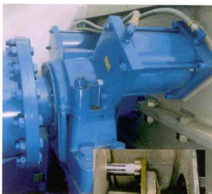
Pneumatic Choke: Automatically controlled, trouble-free pneumatic choke provides lock-up protection.
