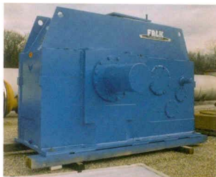
Heavy-Duty Drive Components: Direct-coupled quadruple gear reducer with automatic variable speed.
