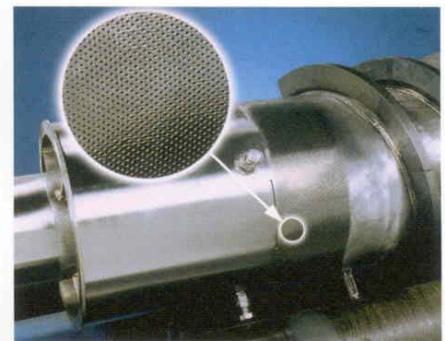
Center Shaft Drainage: Screen on shaft in high pressure section for additional dewatering.
