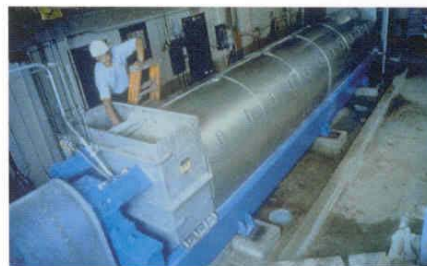
Covers: Removable, 316 stainless steel covers in lift-off sections.
