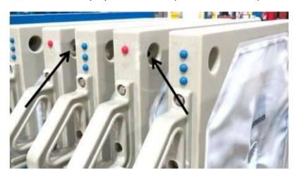
in order from left to right: Rear plate, #3 ported plate, and #1 plate side-by-side
