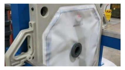
im #Red Button (1B) intermediate plate with visible ports
