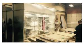
VTLS10 specifications: 10' x 8' x 7' 7000 – 8400 CFM 7HP 1Ph or 3Ph LED light (optional) Pre-wired control panel Custom height and depth Waterborne or Laquer
