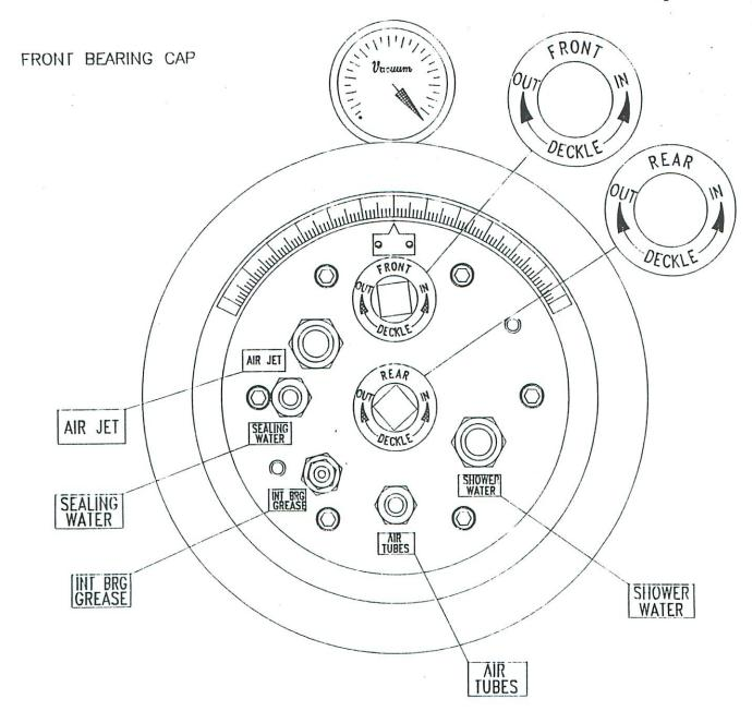
All of the internal connections pass through the front cap and are labeled as follows.
