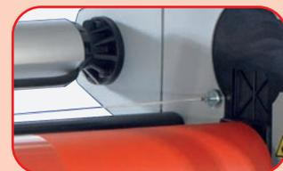
**Shaft** Graduated media shafts. Usable from the storage position
