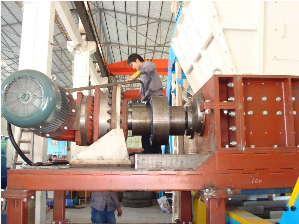
WE ALSO USE A “SPLIT END PLATE DESIGN” WHICH ALLOWS THE CUTTER SHAFTS TO BE REMOVED VERTICALLY AND IN SOME DESIGNS, HORIZONTALLY FROM THE MAIN FRAME OF THE SHREDDER.
