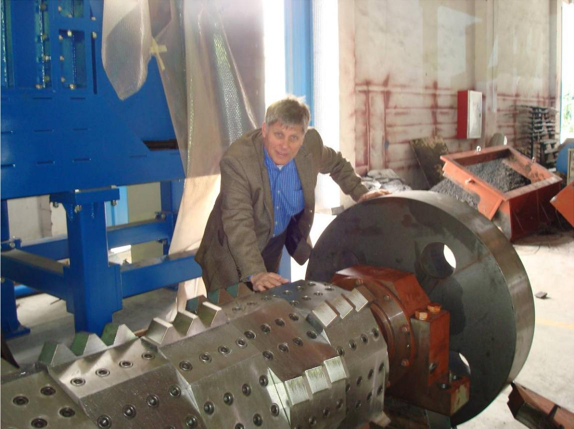
THIS IS THE INTERNAL ROTOR OF A RASPER TYPE MACHINE...
