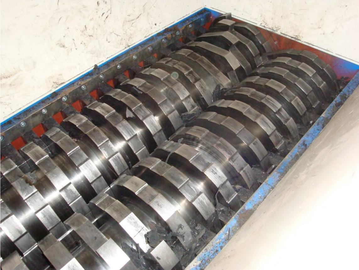
THIS IS A PICTURE OF ONE OF OUR TECHNOLOGIES FOR CUTTERS, THAT ARE USED IN THE PRIMARY AND SECONDARY SHREDDERS, WITH OUR TWO SHAFT MACHINE THAT CUT TIRES, STEEL DRUMS, PALLETS, AND A WIDE ASSORTMENT OF PRODUCTS.....
