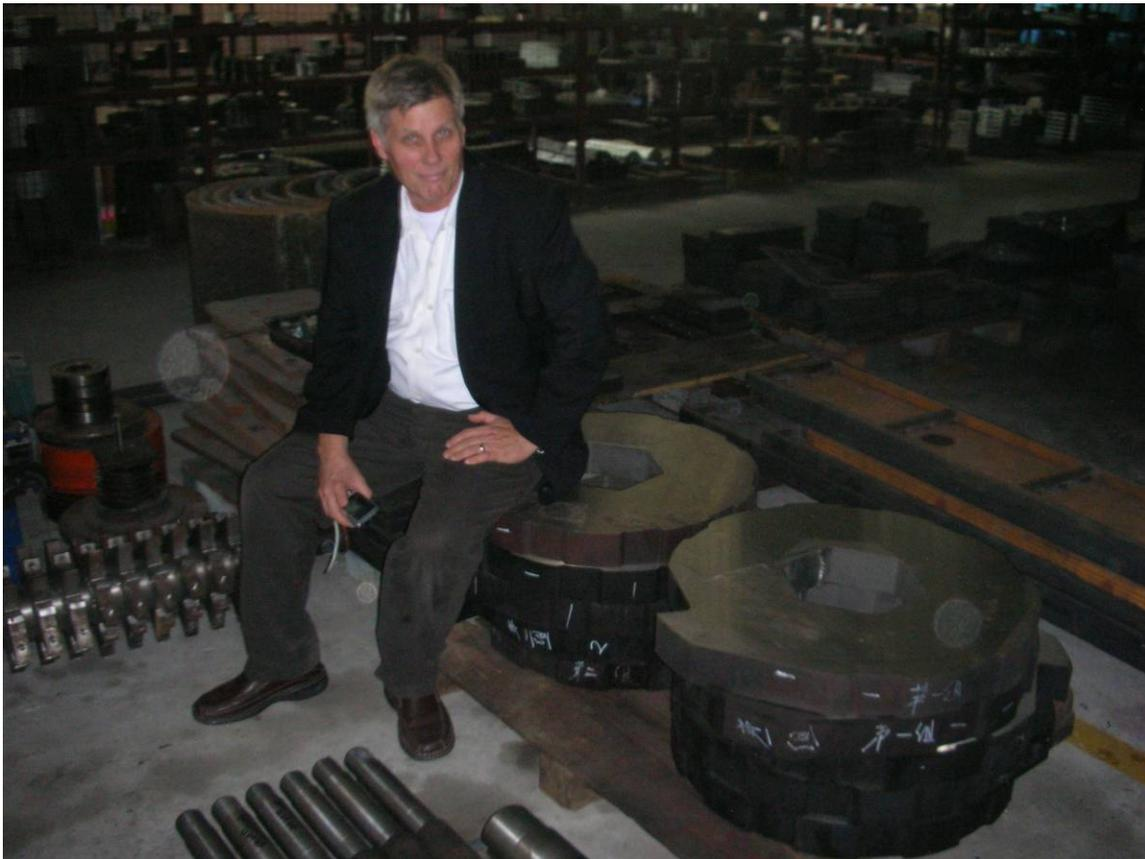
THE PICTURE ABOVE SHOWS THE 34" DIAMETER CUTTER WITH HEX SHAFT DESIGN, THAT YOU WILL FIND IN MANY OF OUR STANDARD PRIMARY SHREDDERS....
