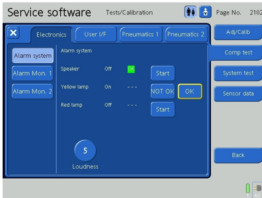
Fig. 82 Alarm System (Page No 2102)
