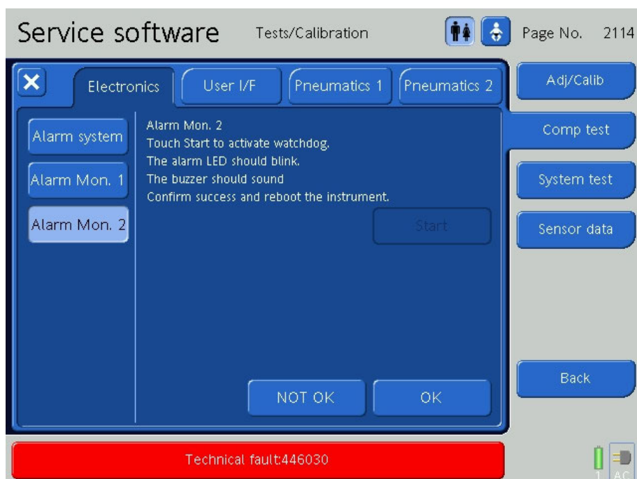
Fig. 98 Alarm monitor test 2 (Page No 2114), Watchdog activated
