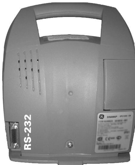
The location of the RS 232 port on rear side of the GE DINAMAP ProCare 100 Series
