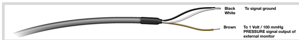
Figure 5-2: External Pressure Interface Cable
