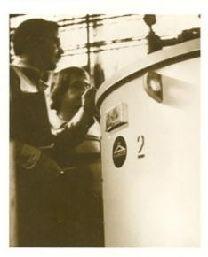
Weyerhaeuser utilizes five White Water Filters with 150-mesh screens to process more than 4 million gpd of white water on the mill's two paper machines. The fine mesh screening recovers fiber particles down to 105 microns in size; the recovered particles are then recycled to the primary fan pumps on the two machines. Screened effluent flows from the White Water Filters to filtered water tanks and from there is recycled to the machine showers.
