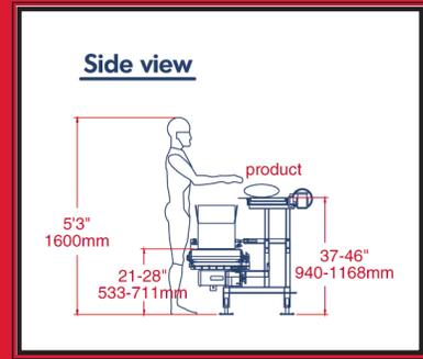
Combi Packaging Systems is the first equipment manufacturer to provide an ergonomic solution for hand packing. Ideal for food packing applications requiring inspection before packing; packing products of variable sizes where total automation is impractical; irregular shaped items that don't lend themselves to automation; or applications where you need more than a stand-alone case erector but less than total automation.
