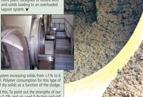
Secondary (WAS) sludge thickening system increasing solids from <1% to 6 to 8%+ prior to hauling for disposal. Polymer consumption for this type of application is typically 4 to 9 lbs/ton of dry solids as a function of the sludge.
