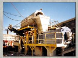
MDS in de-inking sludge thickening service, prior to screw press. The advantage that the MDS delivers in dryer solids was required to meet with the dry solids required from the press (50%+).
