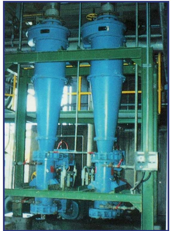
pictured above: Krebs High Density Stock Cleaners removing dense contaminants from paper pulp.
