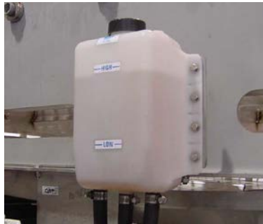
1 gal. H.P.D.E. Reservoir
