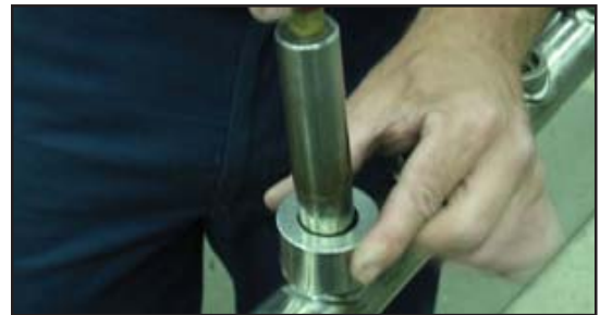
Fig. 4, drive ring in place
