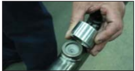
Fig. 3, place tapered collar
