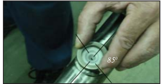
Fig. 2, place the nozzle
