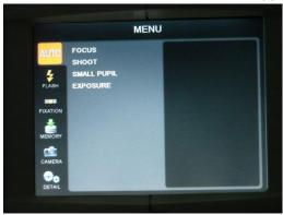
Using the arrows on the control, panel on the right, move the cursor to "Exposure" and set it to "On".
