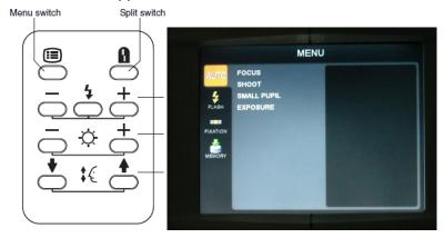
Press the button on the joystick for 10 seconds and the service menu will appear:
