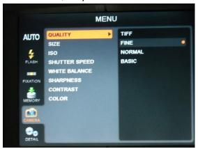
Move one line down to "Size" and select "8M pixel (3264x2448)".
