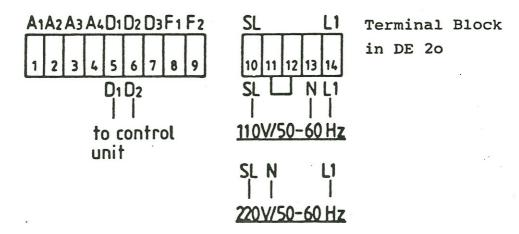
The voltage supply is to terminals N and L  $\mathbf 1$  . Earth is to terminal SL .
