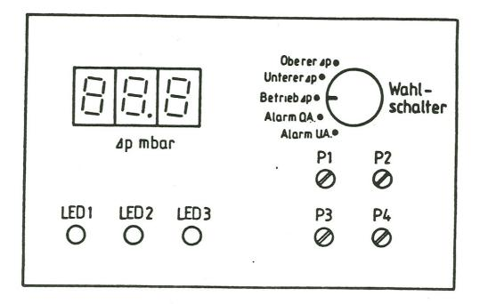
On supplying mains power, the display illuminates and shows O mbar if the fan of the filtering plant is not in operation.
