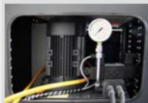
Dual-circuit hydraulic unit in cabinet base
