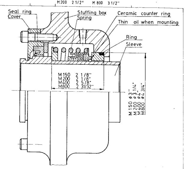
Mount ceramic counter ring with o-ring into stuffing box. Lubricate ceramic counter ring and sleeve with thin oil and mount shaft seal parts around sleeve. Glue carbon ring onto rubber bellow. Clean bellow part before glueing. Sleeve and bellow are to be mounted into stuffing box before glue dries. After this mount seal ring onto upper end of sleeve and mount cover by means of screws. Let bellow and carbon ring set for 30 mins before opening seal water valve or starting motor.
