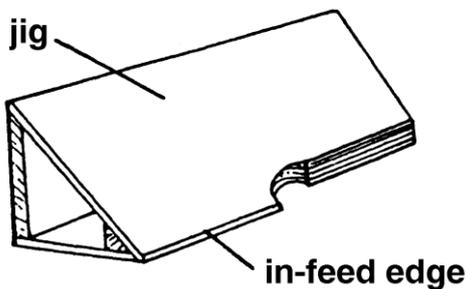
To perform a bevel-edge cut, the in-feed edge of the jig is placed against the infeed fence and clamped to the table as shown in Fig. 31. The outfeed fence is moved forward as necessary to compensate for the cut.
