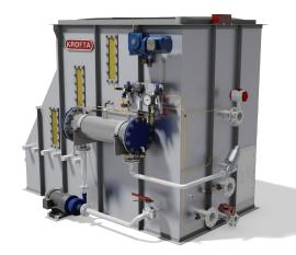
The Krofta Technologies, LLC MULTIFLOAT (MF) is a rectangular DAF unit engineered to be installed in a wide variety of industrial or municipal applications. The unit can be configured vertically (MFV) or horizontally (MFH) to accommodate available space. The all stainless steel rectangular units are offered in 20 standard sizes from 50 – 1,500 gpm capacities.
