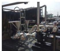
Portable, skid-mounted 90-barrel self-sufficient mixing plants, each equipped with two engines and two pumps, designed for various mixing applications in frac plug drill outs, coil tubing, snubbing, stimulation, workover and blending small batch drilling muds and brines as well as other drilling and completion fluids applications.
