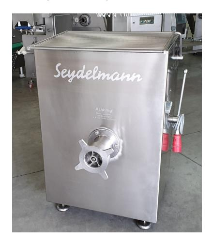
114 mm hole plate diameter Almost completely made of solid stainless steel 2-speed working worm
