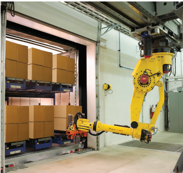
Ceiling mounted M-900 i A/350 unloading trucks.
