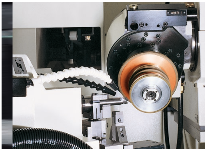
The 2 wheel arbors with up to 8 grinding wheels
