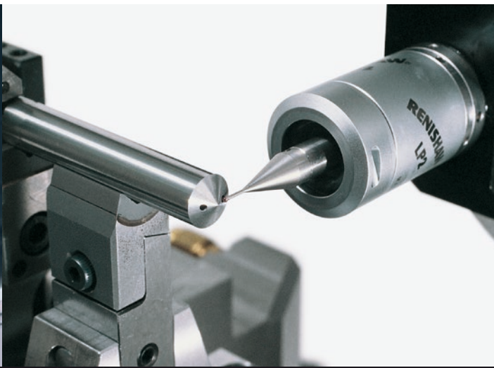
3D probe locating blank with coolant channels
