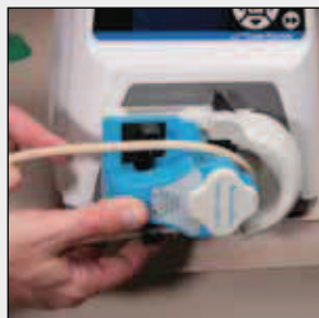
2. Place tubing over rollers and through retainers.
