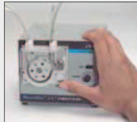
3. Lift occlusion bed and close latch; locking occlusion bed in place.
