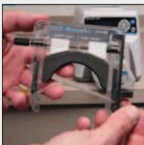
1. Select tubing, load tubing into cartridge, and set tubing retainers.
