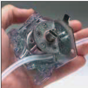
1. Disassemble pump head. Load tubing.
