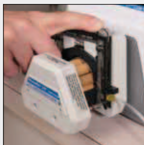
2. Snap cartridge into place on pump head.
