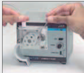
2. Hook left-side tubing stop to the top of the left-side retainer slot. Stretch tubing around rollers and hook right-side stop to the top of the right-side retainer slot.
