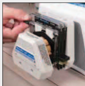
3. Adjust occlusion using index scale on cartridge.
