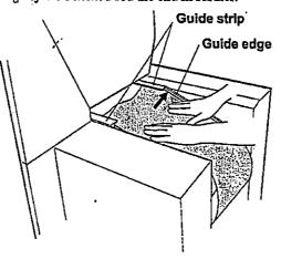
When the strip has been fed in around 100 mm, the first pressure roller will be lowered and will hold the strip against the stationary drive belt. (This presupposes that automatic retention of the paper has been selected with the Paper button in the basic image of the PC program.)
