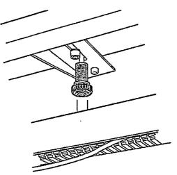
If better access is required, release the socket screws fully, to enable the casing to be pulled forward and then lowered. Note that all doors must be closed or removed to enable the casing to be lowered.
