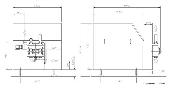
Available up to 400 bar, suitable for CIP and SIP, the Ariete machines can be supplied with all necessary customizations for easy integration in any process line, sanitary or aseptic. The wide range of available materials, the low running speed and linear plunger velocity allow Ariete machines to perform at their best also on abrasive and viscous product.
