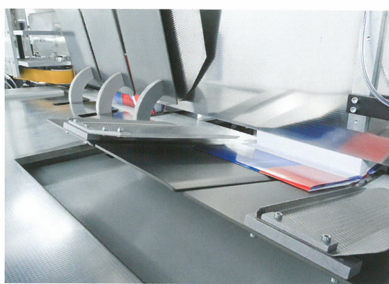
▲ Closing device with precision turn-in elements
