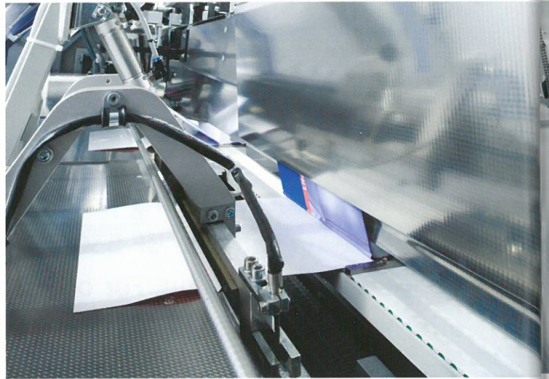
▲ Travelling scoring rails
