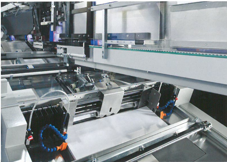
▲ Jacket feeder – separation and infeed
