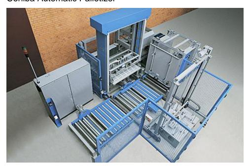
At the end of every print-finishing process the question arises how to economically process and deliver stacks of finished products. An automatic palletizer often is the ideal solution. The Muller Martini Cohiba automatic palletizer is the most efficient choice for any finishing system, for processing adhesive-bound or stitched products delivered from compensating stackers in loose or packaged stacks.
