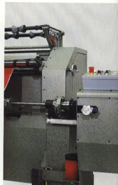
Bearing for the material shaft and operating panel
