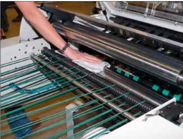
Pressing unit can be opened pneumatically so that the pressing rollers can be cleaned and double sheets can be removed quickly and easily.
