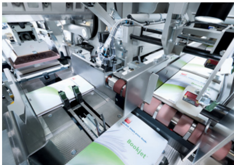
▼ Infeed and cutting of single products
