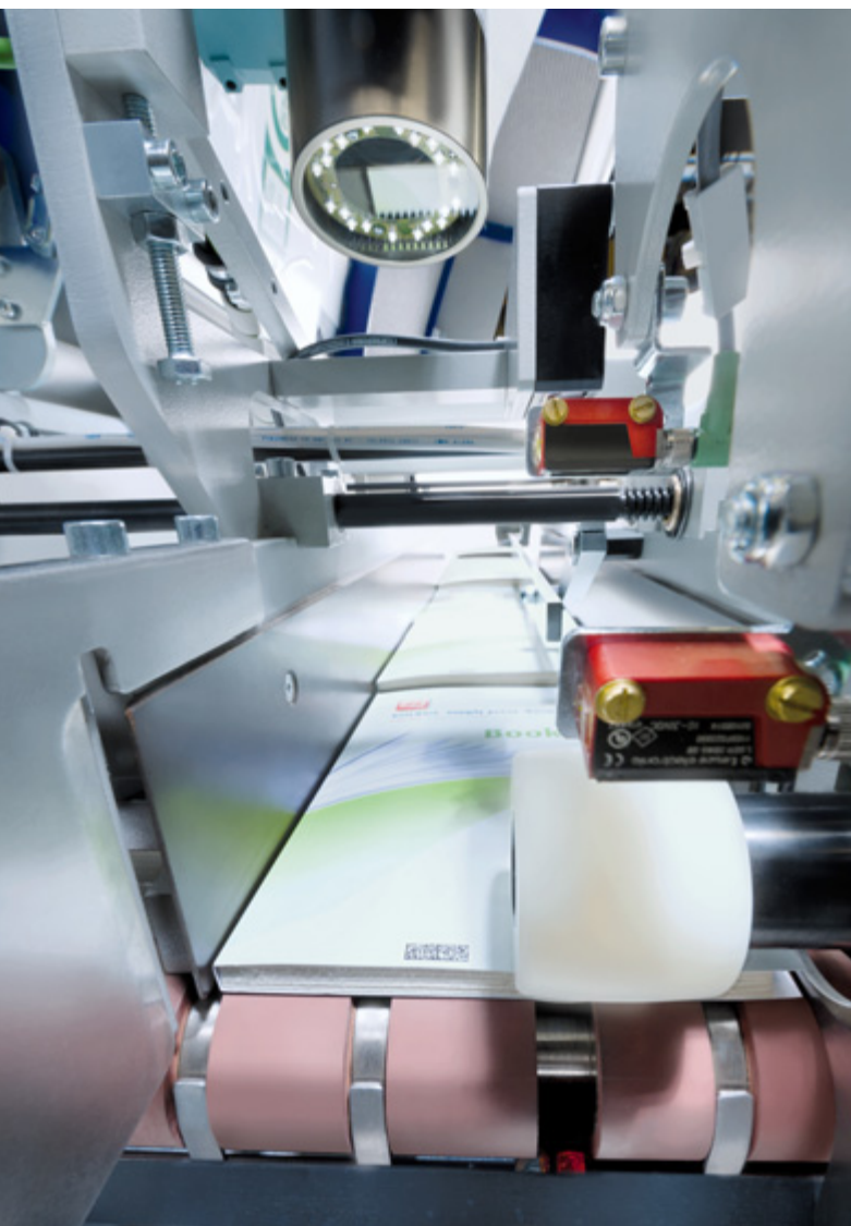
▼ Infeed conveyor with thickness measurement and barcode recognition
