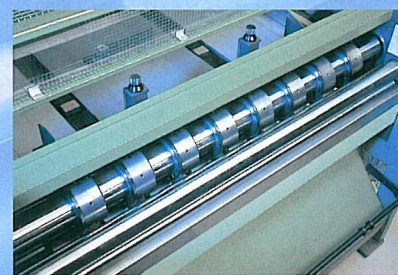
100 mm diameter cutter shafts with solid, divided cutter sleeves for maximum stability
