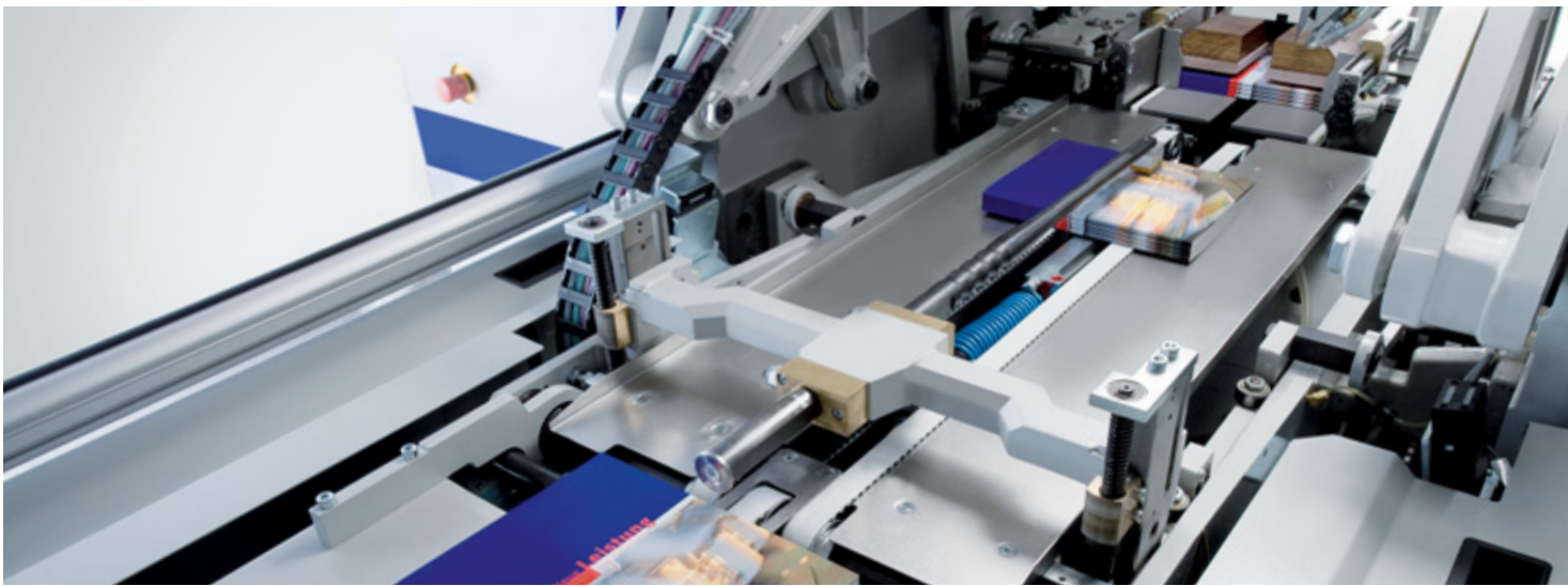
▲ Products are lifted and delivered by grippers
