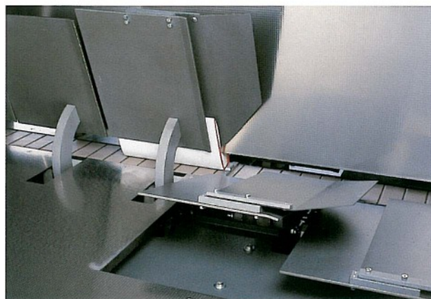
▷ Closing device with controlled folding elements
