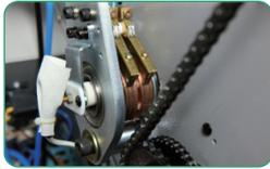
Built-in temperature sensor inside roller
