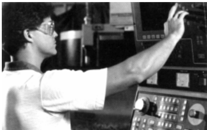
Computer-controlled equipment like this simplifies the process of drilling coil headers.
