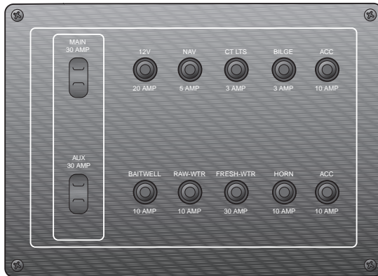
TYPICAL BREAKER / FUSE PANEL
