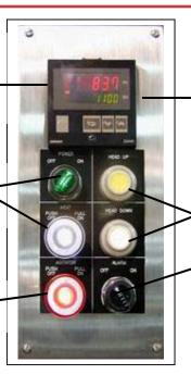
Digital temperature control – Enter your required temperature set-point on the control panel ... FireMixer takes batch up to this temperature and then "cycles" heat on and off to maintain the set-point temperature.
