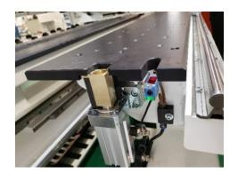
The stop is strong design to offer stable alignment. Besides, the sensor can measure the workpiece X length. The air blow will clean the dust on the sensor.
