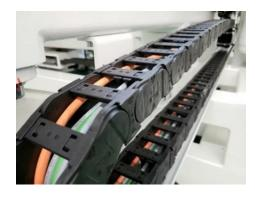
High-quality drag chain used to drag and protect electric wire and air tube during movement of each axis for longer service life.
