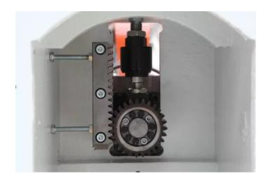
Movement of pressure beam by precise rack and pinion on both sides.
