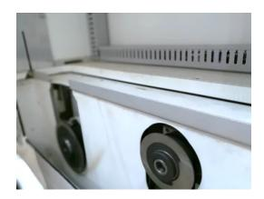
The design prevents saw carriage from struck due to small work piece dropping, hence guarantees the stable working of saw carriage.
