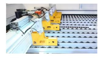
Accurate and smooth movement of feeding unit is ensured by 2kw servo motor and long rack and pinion on both sides. Gear box with German brand.
