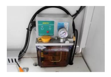
The automatic lubrication system greases the main components automatically that reduces the need of maintenance by operators.
