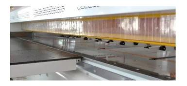
Piano type dust cover provides a completely enclosed blade guard and prevents flying dust and chips.
