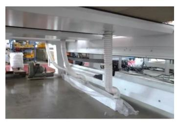
Separate 3 pipes connected to 3 float tables with a 2.2kw air blower beneath the table supplies sufficient air.
