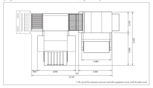
■ Layout for PlateRite Ultima 16000 with MA-L16000N (six-cassette autoloader type) [units: mm]
