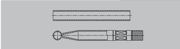
Tube with differing wall thickness produced by swaging over a mandrel, with external splines on both ends.
