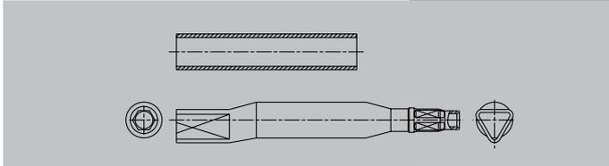
Tube produced by plunge swaging in several stages.
