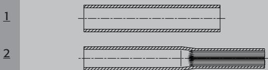
Tube produced by infeed swaging operation over a profiled mandrel in one operation.
