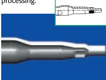
**8 Turning:** The material must be allowed to flow freely in one axial direction during the forming process. The excess material is removed by an end facing process, which is carried out together with simultaneous end chamfering and turning of circular grooves.
