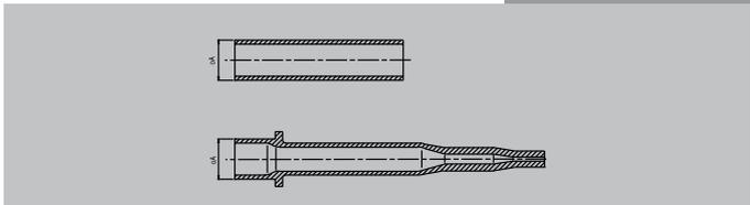
Example of a sophisticated internal profile produced by swaging over a mandrel in one operation.
