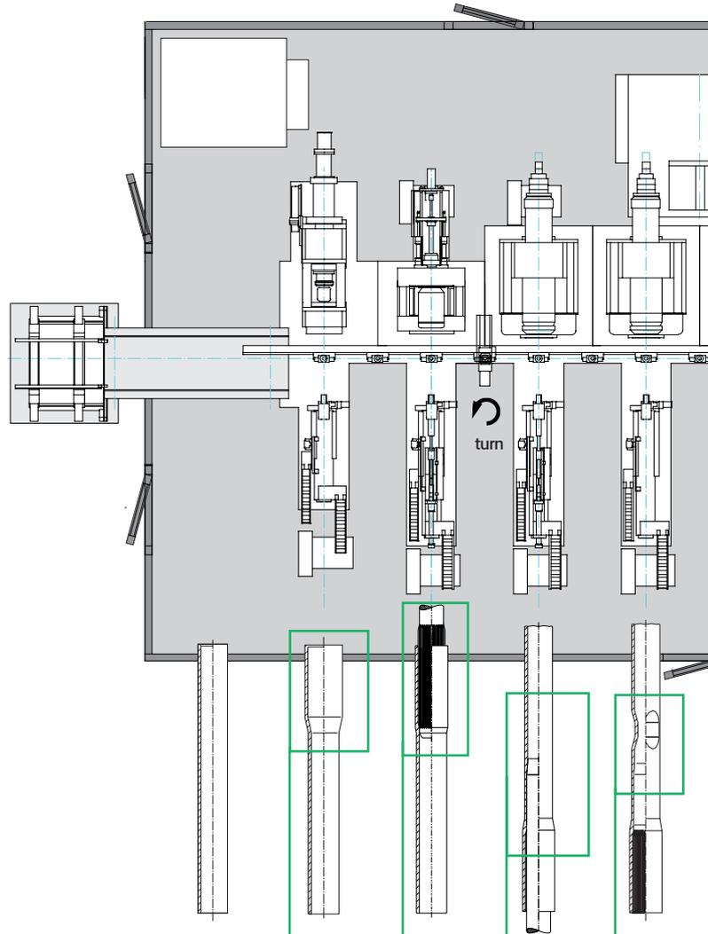
**1 Expanding:** Production of the pre-diameter for the internal spline on a hydraulic axial forming machine.
