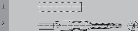
Tube produced by infeed and plunge swaging operations.
