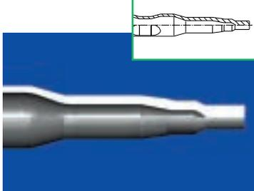
**7 Spline forming:** Production of the external spline on a hydraulic axial forming machine. The high spline quality allows direct assembly of the component without further processing.
