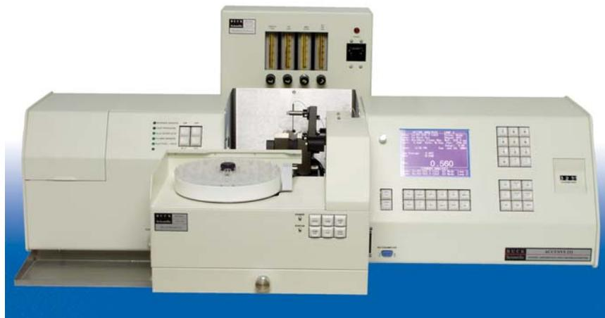
The 210/211 can initiate multistep sequences with alternate gas purging for fully optimized STGFAAS.
