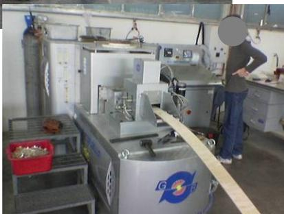
The horizontal continuous casting furnace **LOGIC**, with induction heating system, has been conceived to produce wires, plates, tubes and customized special sections.
