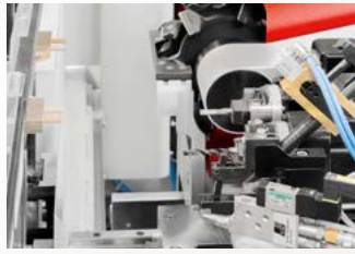
Routing for French Cut frame joints
