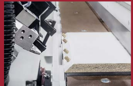
Tiltable drilling and dowel insertion unit (0° and 45°)
