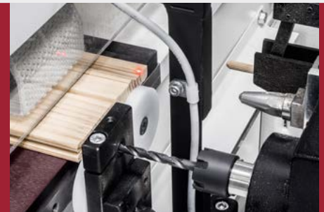
Automatic detection of stock width
