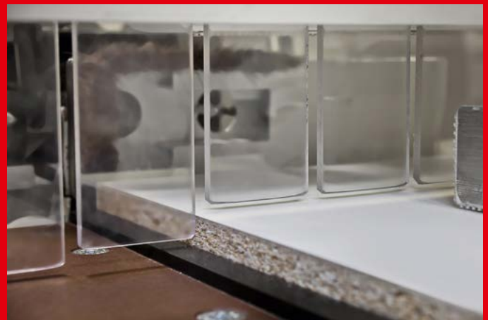
A safety curtain with transparent lamellas and a memory function protects against inadvertent entry into the danger zone
