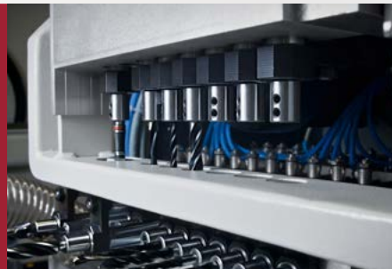
Customized drilling station with seven vertical and ten horizontal drilling spindles
