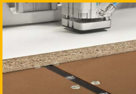
The center fence can be lowered manually to accommodate large workpieces
