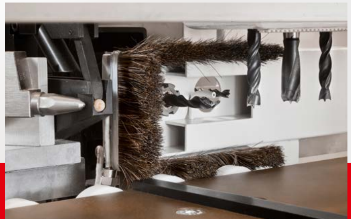
Drilling and dowel insertion station
