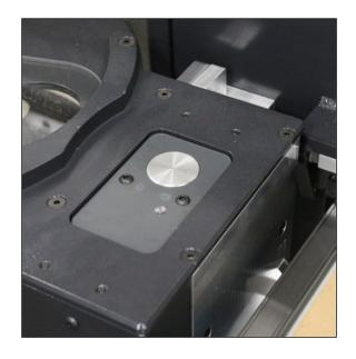
The tool length sensor is used to automatically measure the length of a tool and create an accurate tool length offset. This saves you time and ensures precise and consistent cutting depths with all tools.
