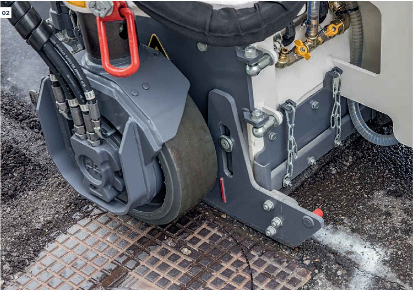
01 - 02 The electronically controlled travel drive makes high-precision milling possible - such as around road installations, for example.
